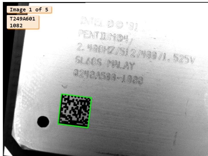
Figure 2.1: Visualization of the result: surrounding XLD contour of the symbol and decoded string.
