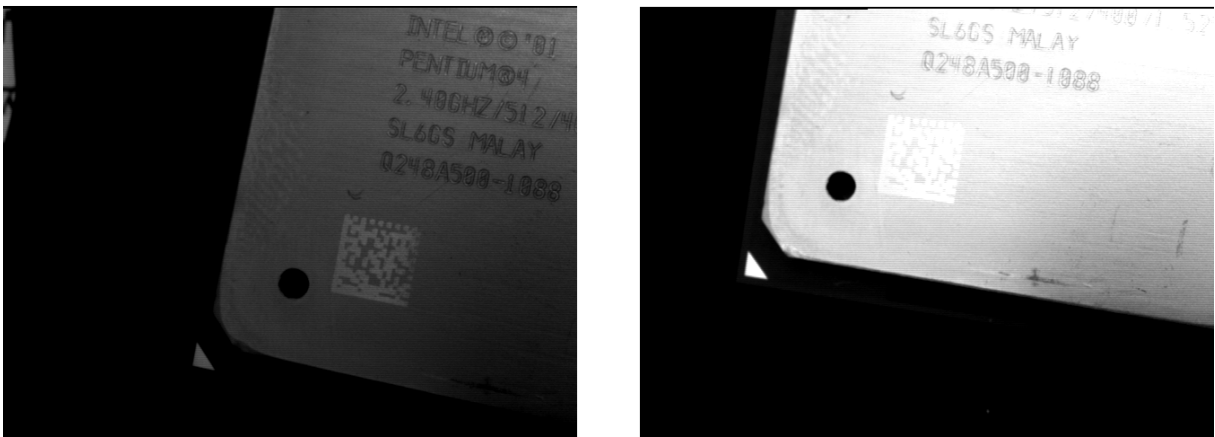
Figure 3.2: Images with different contrast values for training the 2D data code model.
