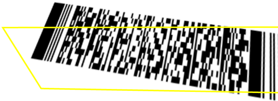
Figure 5.10: The symbol candidate is related to the stop pattern and does not fit the actual symbol outline.
