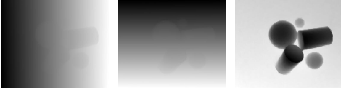
Figure 4.16: Height data used for 3D primitives fitting: (from left to right) X, Y, and Z image.
