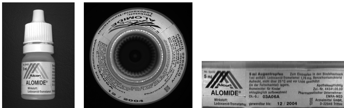
Figure 2.22: (left) Side view of the vial that should be inspected, using a regular lens. (middle) Top view using a hypercentric lens. (right) Unrolled surface of the label, after camera calibration and mapping.
