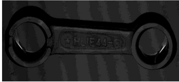
Figure 6.18: Result of uncalibrated sheet-of-light measurement: score image ( score_type set to 'width', i.e., bright parts indicate artifacts).
