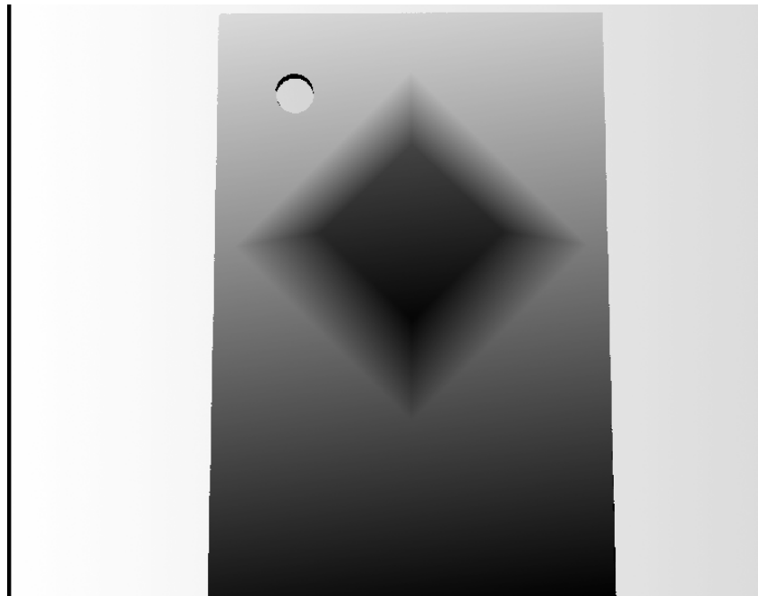
Figure 6.11: Disparity image of the 3D calibration object.
